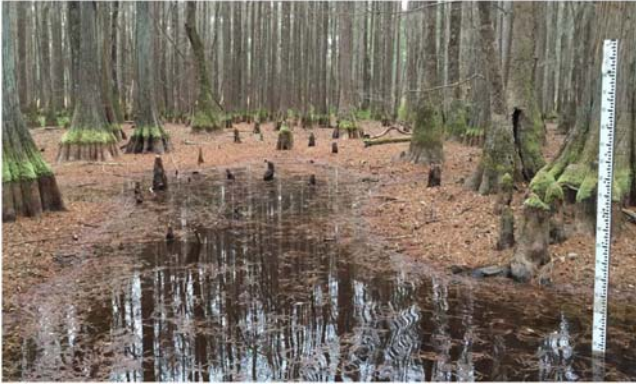
FIGURE 3.7 Staff gauge used to measure water level in a depressional subtropical forested wetland. Photo credit: James B. Deemy.
