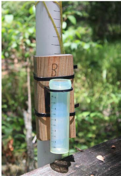
FIGURE 3.6 Plastic rain gauge installed on a small barrier island freshwater depression. Quantification of the rainfall-stage and water-quality relationship is possible when combined with a stilling well containing pressure transducers and a specific conductance probe. Photo credit: James B. Deemy.
