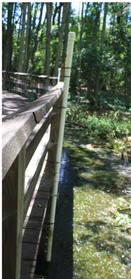
FIGURE 3.9 Stilling well installed in a small, semiisolated, subtropical, freshwater, depression wetland on St. Simons Island Georgia, United States. Photo credit: James B. Deemy.
